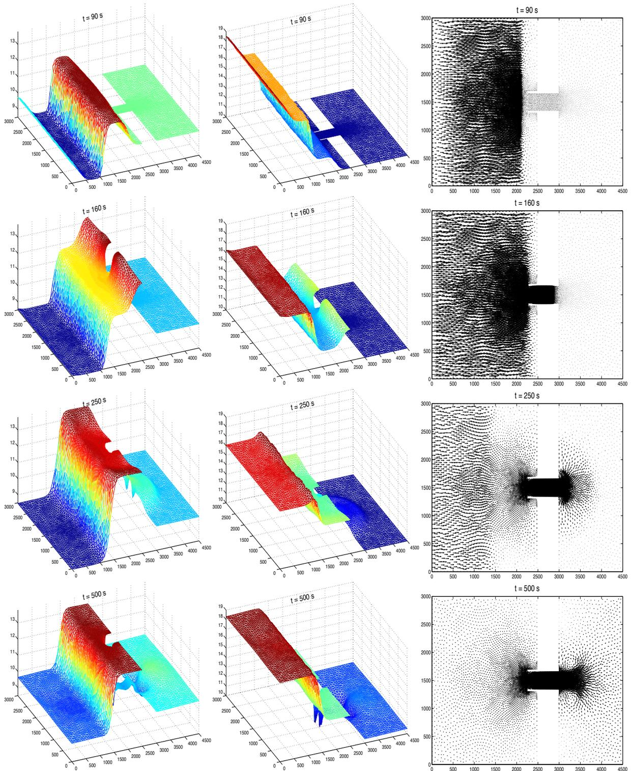
Figure 6: Water height  $h$  (first column), water density  $\rho h$  (second column) and velocity vectors (third column) for the idealized inlet system at four different simulation times. From top to bottom  $t = 90, 160, 250$  and  $500$  s.
