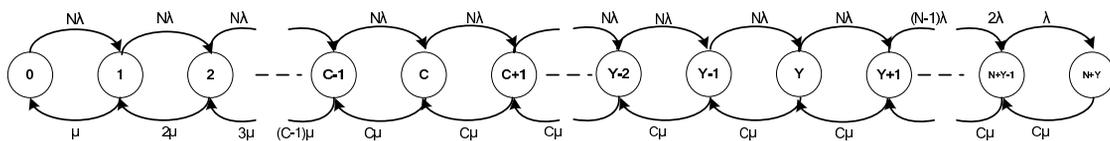
Figure 6: Transition diagram of the repairman model.
