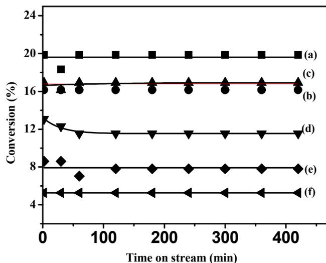
Fig. 9: Propane conversion versus time on stream at 425°C over 10Ni<sub>1-y</sub>Nb<sub>y</sub>/CaHAp for (a) y = 0.05; (b) y = 0.1; (c) y = 0.15; (d) y = 0.2; (e) y = 0.3; (f) y = 0.4.
