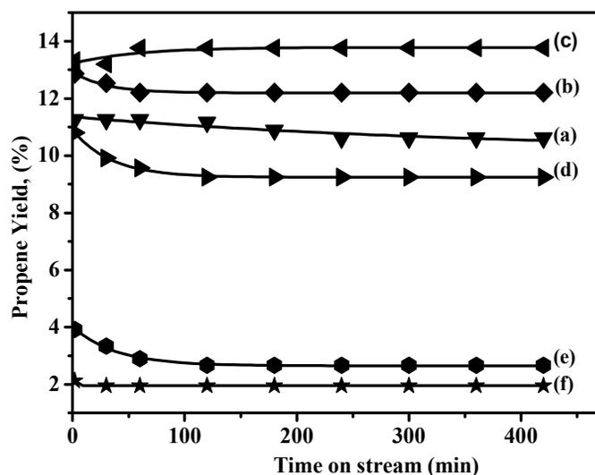
Fig. 10: Propylene yield versus time on stream at 425°C over 10Ni<sub>1-y</sub>Nb<sub>y</sub>/CaHAp for (a) y = 0.05; (b) y = 0.1; (c) y = 0.15; (d) y = 0.2; (e) y = 0.3; (f) y = 0.4.
