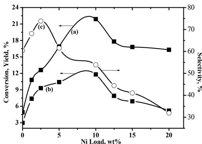
Fig. 8: Propane conversion (a), propylene yield (b) and selectivity (c), versus nickel load over  $x\text{Ni}/\text{CaHAp}$  at  $425^\circ\text{C}$ .
