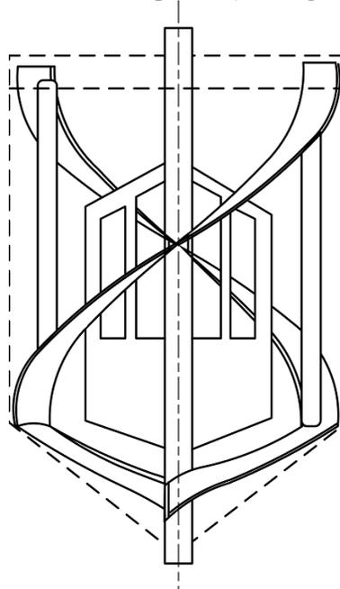
Figure 11 : Superblend coaxial mixer.
