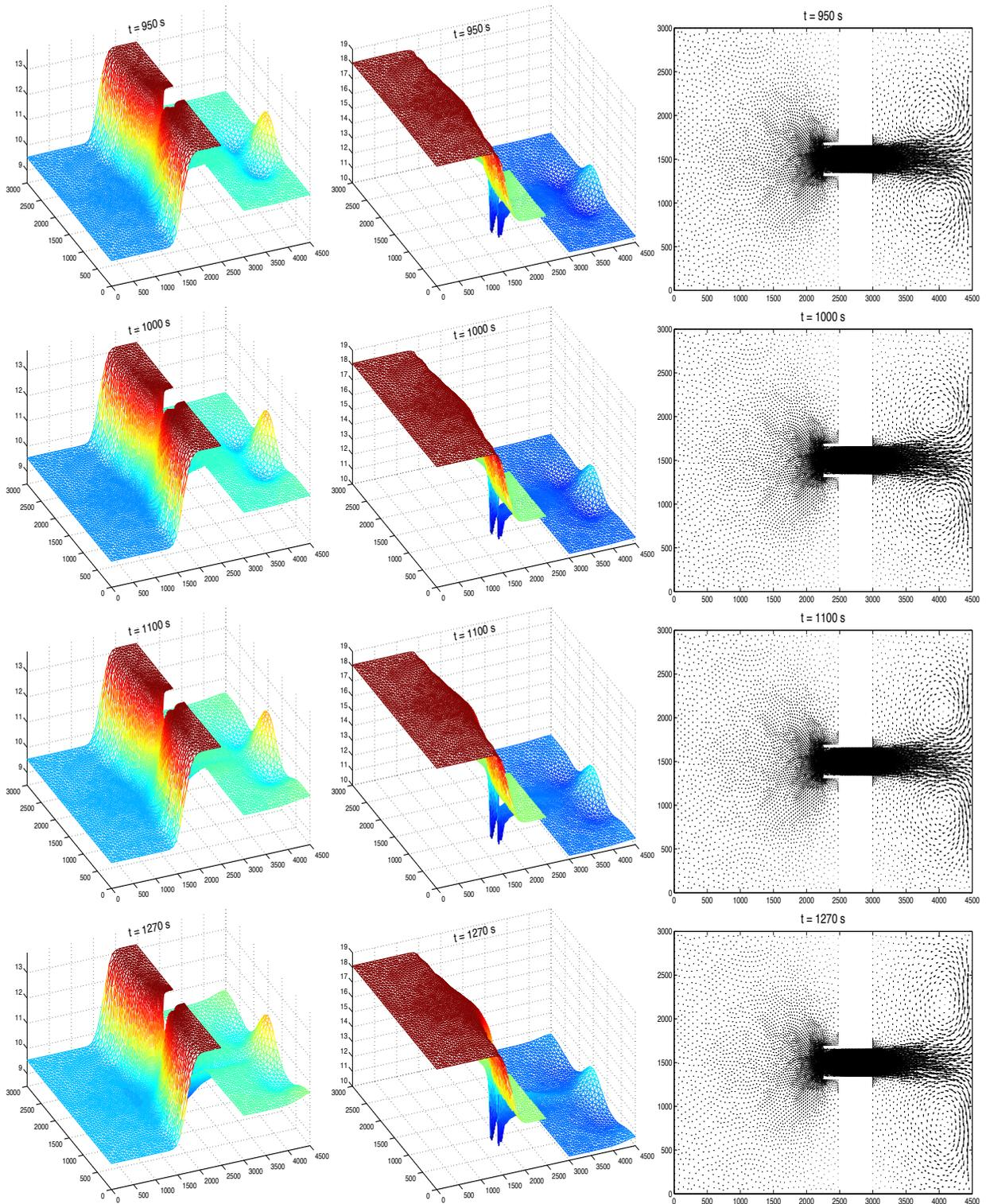
Figure 7: Water height  $h$  (first column), water density  $\rho h$  (second column) and velocity vectors (third column) for the idealized inlet system at four different simulation times. From top to bottom  $t = 950, 1000, 1100$  and  $1270$  s.
