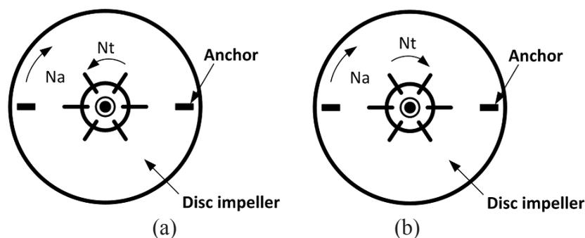
Figure 9: Rotating modes: (a) Counter-rotating; (b) Co-rotating. (21)
