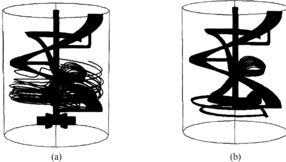
Figure 6: Dispersion pattern: (a) Induced by the dual impeller; (b) Induced by the helical ribbon only (18).
