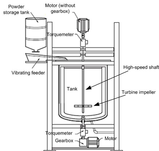
Figure 7: Coaxial mixer with scraping and dispersing impellers (20).
