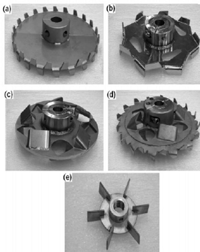
Figure 8: Dispersing turbines: (a) Cowles; (b) Deflo; (c) Sevin; (d) Hybrid turbine; (e) Rushton turbine (21)
