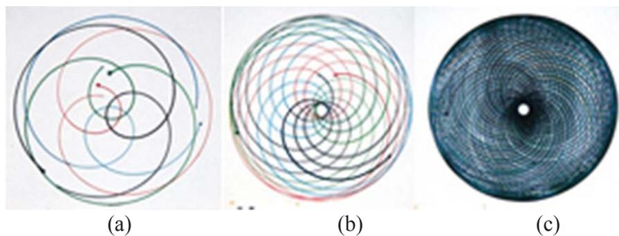
Figure 13: Cross-section flow fields observed with planetary mixers: (a) In the beginning; (b) after one revolution; (c) after several revolutions. (27)
