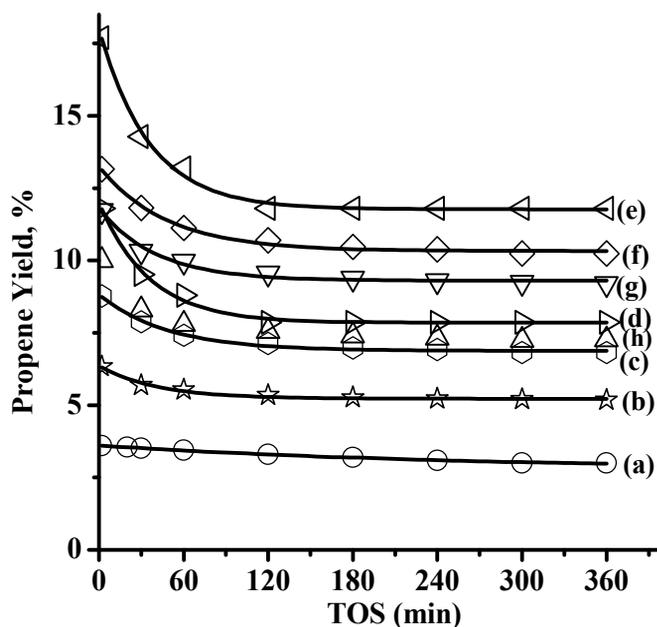
Fig. 7: Propylene yield versus time on stream at 425°C on xNi/CaHAp catalysts where: (a)  $x = 0$ ; (b)  $x = 20$ ; (c)  $x = 15$ ; (d)  $x = 12$ ; (e)  $x = 10$ ; (f)  $x = 5$ ; (g)  $x = 2.5$ ; (h)  $x = 1.25$ .
