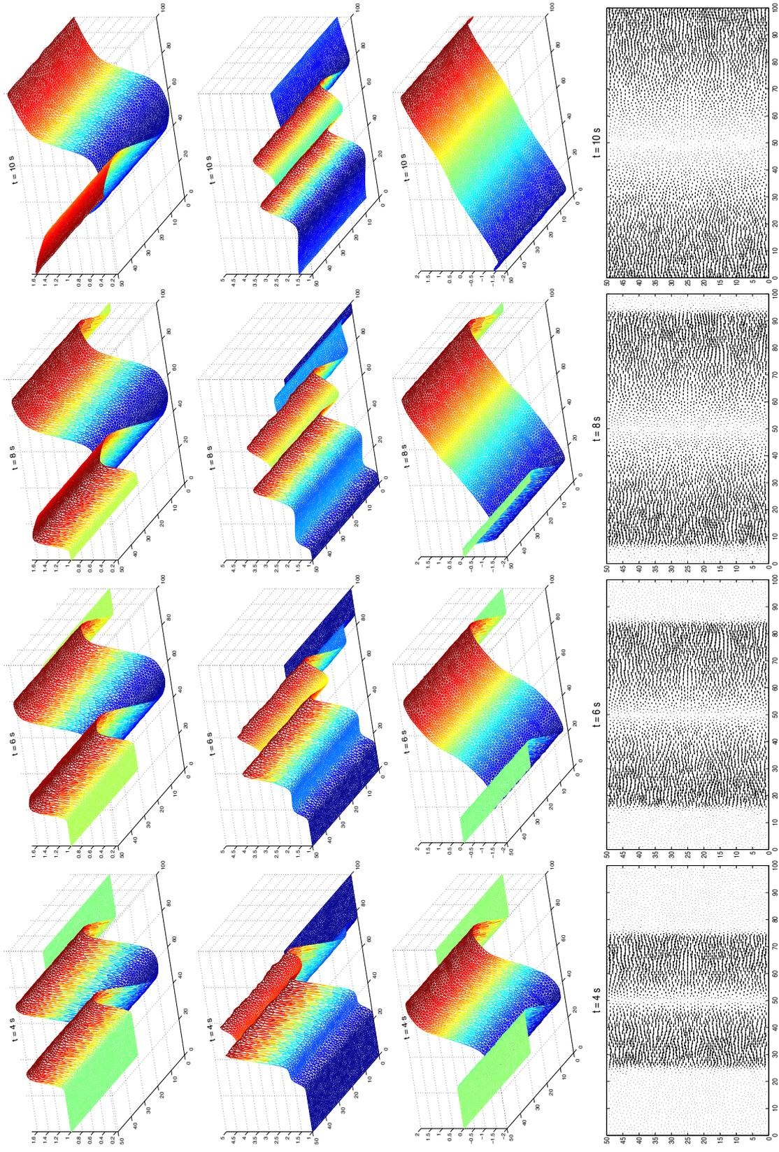
Figure 5: Water height  $h$  (first row), water density  $\rho h$  (second row),  $x$ -velocity  $u$  (third row) and velocity vectors (fourth row) for dam-break with double density discontinuity at four different simulation times. From left to right  $t = 4, 6, 8$  and  $10$  s.
