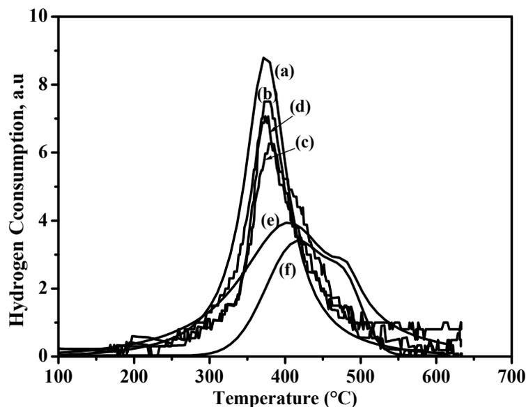
Fig. 5: Temperature Programmed Reduction profiles of  $10\text{Ni}_{1-y}\text{Nb}_y/\text{CaHAp}$  with: (a)  $y = 0.05$ ; (b)  $y = 0.1$ ; (c)  $y = 0.15$ ; (d)  $y = 0.2$ ; (e)  $y = 0.3$ ; (f)  $y = 0.6$ .
