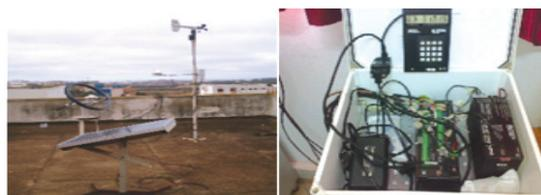
Fig. 1. Meteorological station with the data logger Campbell CR10X
