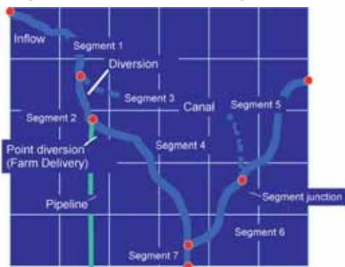
Figure 15. Example of a streamflow routing network with main streams, tributaries, diversions, and connections to surface-water deliveries to the Farm Process in MODFLOW.
