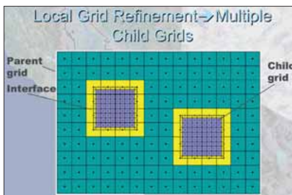
Figure 19. Example of Relation between regional (parent) and more detailed, embedded (child) model grids using LGR in MODFLOW.
